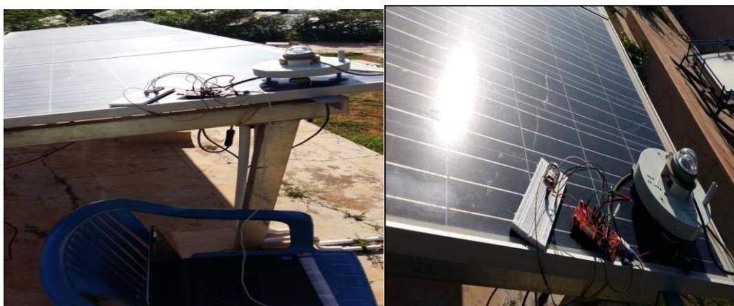
**Figure 5.** Experimental Setup of Solar PV Monitoring System
