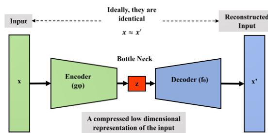
**Figure 6.** Structure of Autoencoders for Anomaly Detection
